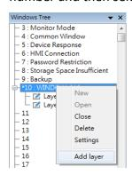
The following is an example of creating a layered window: Place a Bit Lamp object in Layer 1 and a Numeric object in layer 2.
